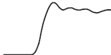
Figure 7: Signal with a long ground lead
